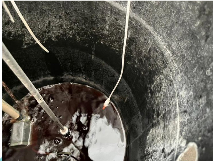
Gambar 4.5 Implementasi Modul Sensor TDS Analog
