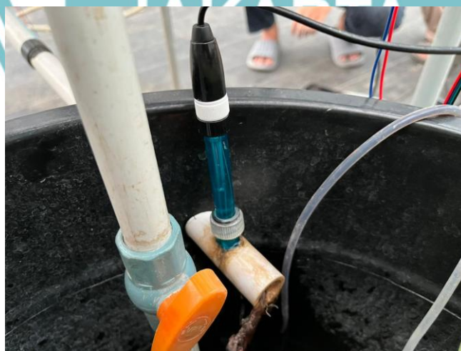
Gambar 4.6 Implementasi Modul Sensor pH-4502C
