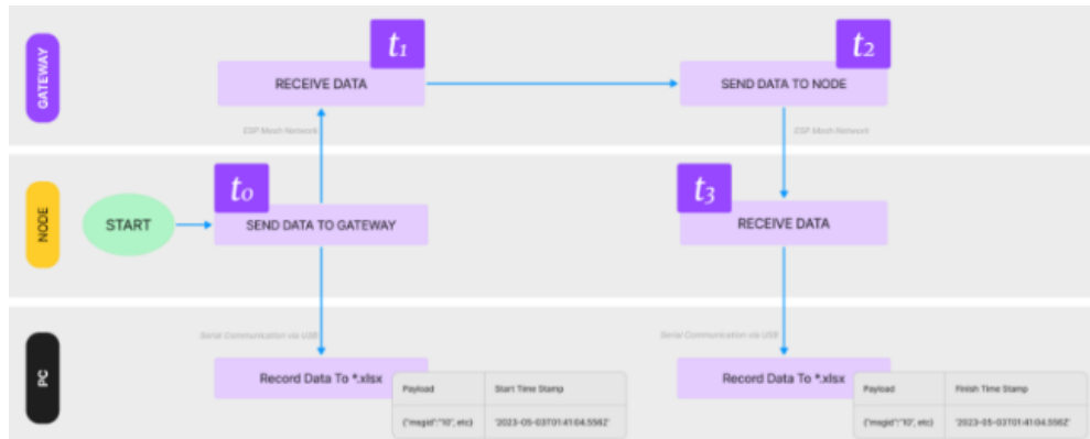
Gambar 4.37 Alur pengukuran full trip data latency
